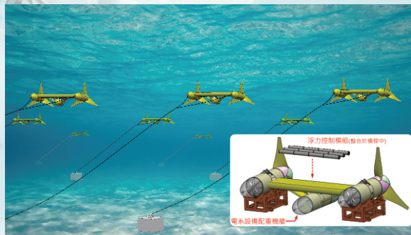
Schematics of the ocean-current power generator and the subsea power generation array.
